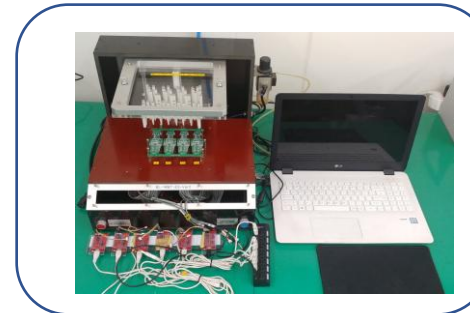
PBA DOWENLOAD 및 TEST JIG
